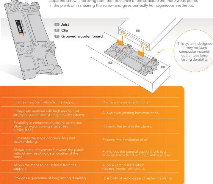
The Softline® fixation system allows free circulation of air and movement between the planks without any resulting deterioration of the wood.
